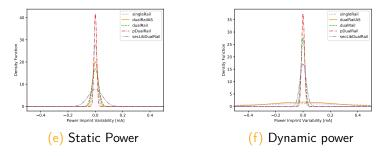
Selected density functions (PDF) for power imprints of all implementations - a narrower curve means a better protection.
