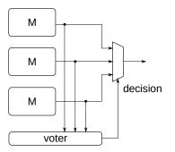
Conceptual scheme of an error-correcting Triple-Modular redundancy (TMR)
