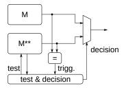
Conceptual scheme of proposed error-correcting Time-Extended Duplex (TED)
