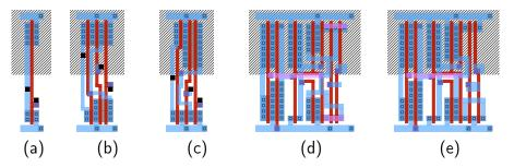
Standard cells in TSMC180nm: (a) INVX1, (b) AND2X1 and
