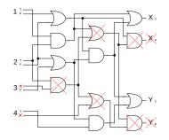
Dual-rail logic circuit derived from the sinle-rail one represents  $\ensuremath{\mathbb{M}^{**}}$
